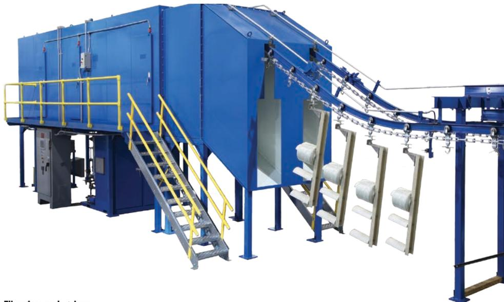
**Fiberglass roving dryer.**
